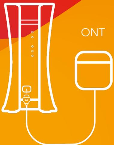
Connect your ethernet cable\* from the ONT on the wall into the red port on the back of your router.
